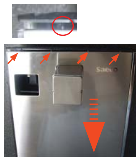
To remove the cover slide downwards and after to the right to release the anchors "see images".
