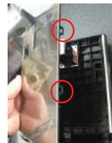
To remove the cover slide downwards and after to the right to release the anchors "see images".
