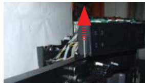
Lift the pin with a screwdriver and remove it through the top of the door.
