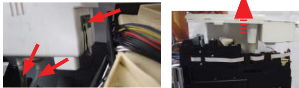
Disconnect all electrical and water circuit connections and remove the top cover.
